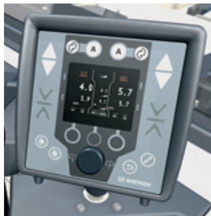
LEVEL PRO PLUS levelling system.
